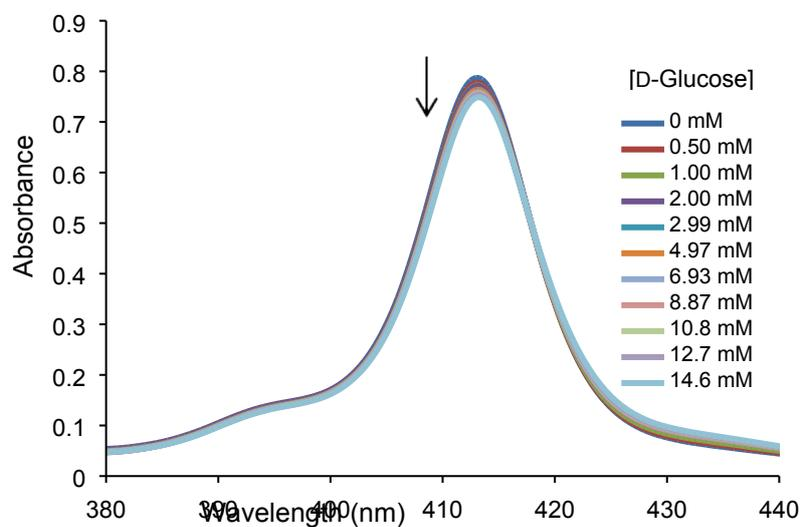
**Fig. S1.** Expansion of the Soret band region of the spectrum ( $\lambda_{\max}$  413 nm) for a titration of TPPS (6.15  $\mu\text{M}$  in water) with D-glucose (0 – 14.6 mM) at constant TPPS concentration.
