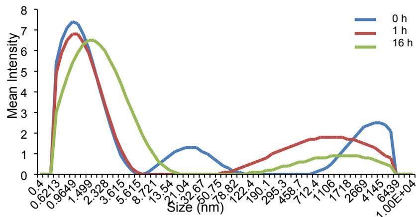
**Fig. S11.** Size distribution and mean intensities for the dynamic light scattering study of TPPS 1 (6.0  $\mu\text{M}$ ) + glucose (600  $\mu\text{M}$ ) in water at 25  $^{\circ}\text{C}$  at 0, 1 and 16 h after sample preparation.
