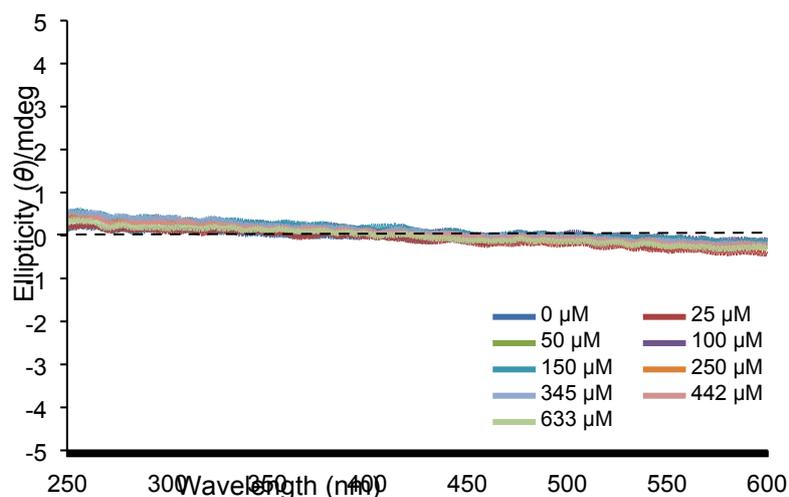
**Fig. S7.** The CD spectra for the addition of D-glucose (100 mM) to TPPS **1** (6.15  $\mu\text{M}$ ) in water-methanol (95:5). The absence of any significant signal argues against a close association between chiral carbohydrate and achiral chromophore.
