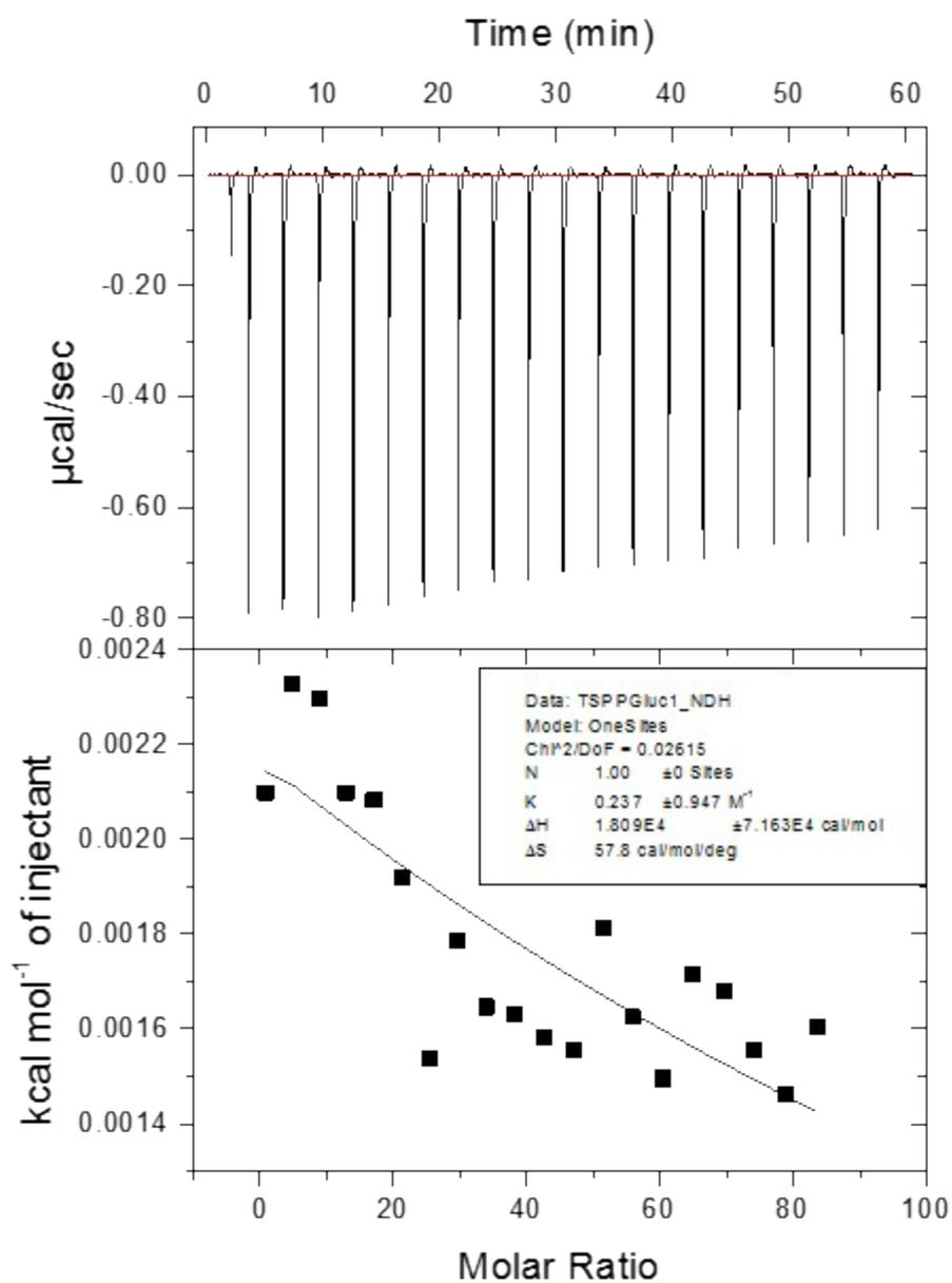
**Fig. S6.** Output from the ITC experiment for the addition of D-glucose (100 mM) to TPPS **1** (0.5 mM) in water. The raw data (top panel) is closely similar to the control titration with no TPPS present, implying that the heat evolved is mainly due to dilution of glucose. The corrected output (lower panel) shows no sign of saturation as expected for complex formation.
