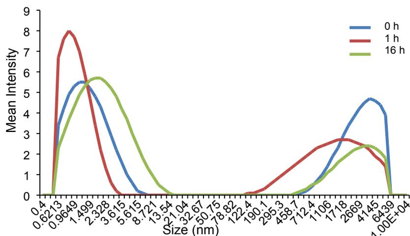
**Fig. S10.** Size distribution and mean intensities for the dynamic light scattering study of TPPS 1 (6.0  $\mu\text{M}$ ) in water at 25  $^{\circ}\text{C}$  at 0, 1 and 16 h after sample preparation.
