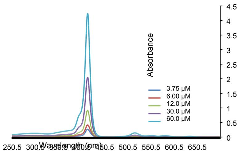
**Fig. S4.** UV-visible spectra for TPPS in water-methanol 95:5 at varying concentrations. Path length = 1 cm. For a plot of absorbance against concentration see Fig. 2.
