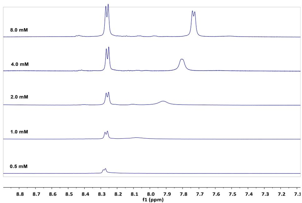
**Fig. S5.** Partial  $^1\text{H}$  NMR spectra of TPPS 1 at different concentrations (8.0 mM diluted to 0.5 mM) in  $\text{D}_2\text{O}$  at 298 K. This experiment serves as a control for the titration of TPPS into glucose (Fig. 3a). The same  $^1\text{H}$  NMR changes are observed in the presence and absence of glucose. They are therefore ascribed to changes in TPPS aggregation state and not to an interaction with carbohydrate.
