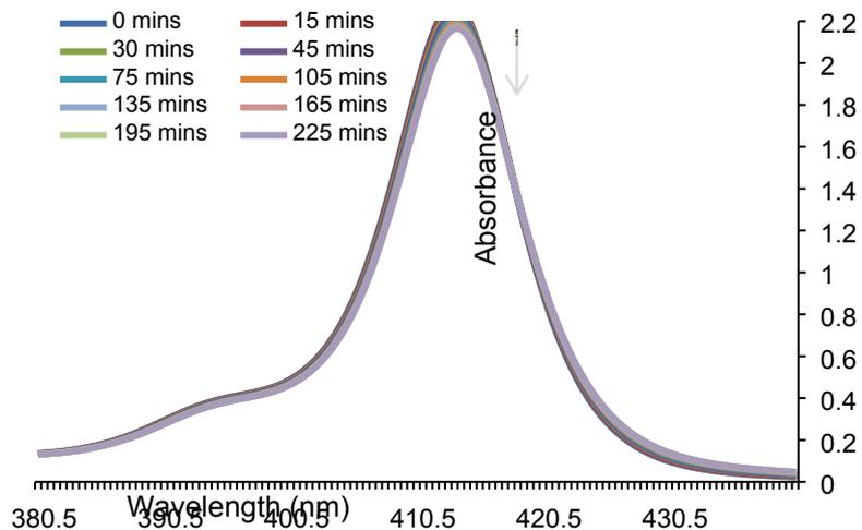
**Fig. S8.** Variation with time of the UV-visible spectrum (Soret band region) of TPPS (6.0 μM) in water. Spectra were acquired between 0 and 225 min after preparation of the sample by dilution from 1 mM aqueous solution.
