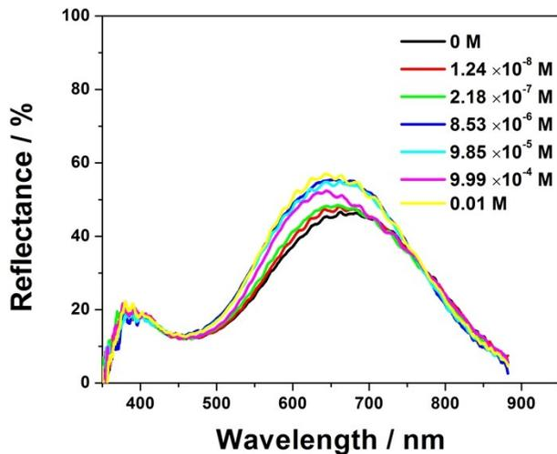
**Fig. S4** Glucose concentration dependence of the hydrogel sensor reflectance measured with a spectrometer in the Littrow configuration, where the diffracted light diffracts back parallel to the direction of the incident light.
