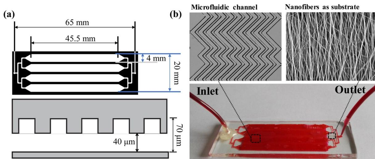
**Figure S6.** (a) The structure and dimension of the designed microfluidic channel. (b) Photograph of the nanofiber-integrated microfluidic chip. Upright and upright panels show the magnified micrograph of the channel and the SEM image of nanofibers.
