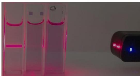
**Fig. S31** Tyndall effect experiments of TPA-S-TPP (10  $\mu\text{M}$ ) in different solvents (from left to right: Toluene, DW, and DMSO) using a red pointer pen.
