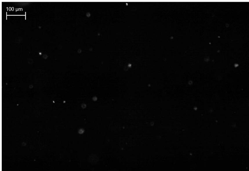
Figure S20: In-line real-time image at T=3.25hr of  $\text{CaCO}_3$  particle development over the filtration time [h] for nanofiltration of high supersaturated effluent. Decreased RBI due to reduced particle concentration resulting from their contribution to cake layer build-up on the membrane surface.
