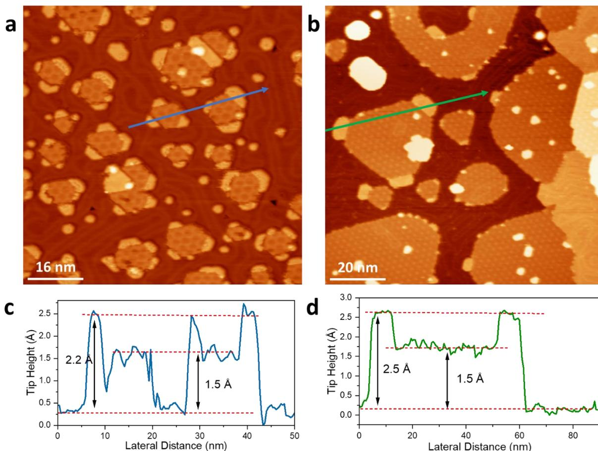
**Fig. S5** STM images of Pd-FeO (a) and Pt-FeO (b) on Au(111). The line profile on Pd-FeO/Au(111) (c) indicates a height of Pd and FeO at  $\sim 2.2$  Å and  $1.5$  Å, respectively, while the line profile of Pt-FeO/Au(111) (d) indicates a height of Pt and FeO at  $\sim 2.5$  Å and  $1.5$  Å, respectively. The heights match literature reports of single-layer thick Pd, Pt and FeO films as observed with STM.<sup>1-3</sup>
