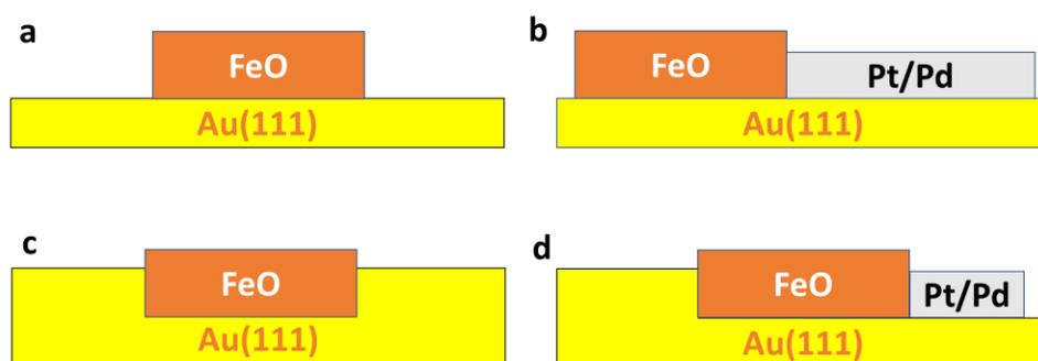
**Fig. S4** Schematic diagram of interfaces in a Pt/Pd-FeO/Au(111) system. (a) Supported FeO with all edges exposed. (b) Supported Pd/Pt-FeO with one type of edge blocked, and the other type exposed. (c) Embedded FeO with all edges blocked by Au. The FeO is embedded into the center of the Au(111) terrace. (d) Embedded Pt/Pd-FeO with both Au-FeO and Pt/Pd-FeO interfaces. The FeO is embedded into the step edge of the Au(111) terrace.
