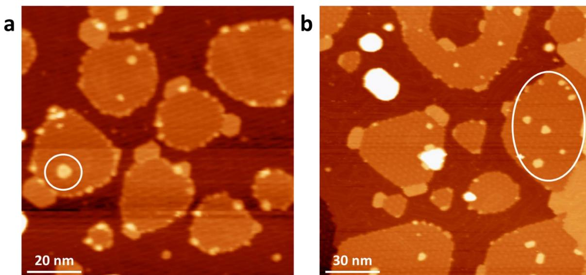
**Fig. S2** (a) STM image of Pt-FeO/Au(111) with a FeO coverage of about 0.4 ML ( $V_{\text{bias}} = 1.6$  V,  $I = 0.3$  nA). (b) STM image of Pt-FeO/Au(111) with a FeO coverage of about 0.5 ML ( $V_{\text{bias}} = 1.6$  V,  $I = 0.2$  nA). White circles mark the Pd located in the interiors of FeO islands.
