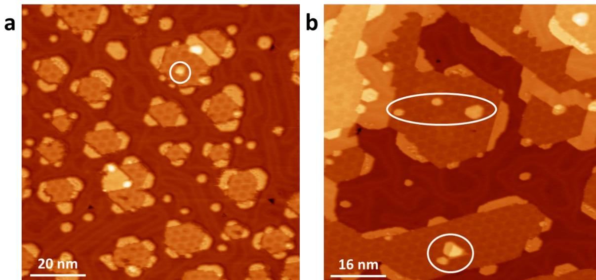
**Fig. S1** (a) STM image of Pd-FeO/Au(111) with a FeO coverage of about 0.3 ML ( $V_{\text{bias}} = -1.7$  V,  $I = 0.5$  nA). (b) STM image of Pd-FeO/Au(111) with a FeO coverage of about 0.5 ML ( $V_{\text{bias}} = -1.2$  V,  $I = 0.3$  nA). White circles mark the Pd located in the interiors of FeO islands.
