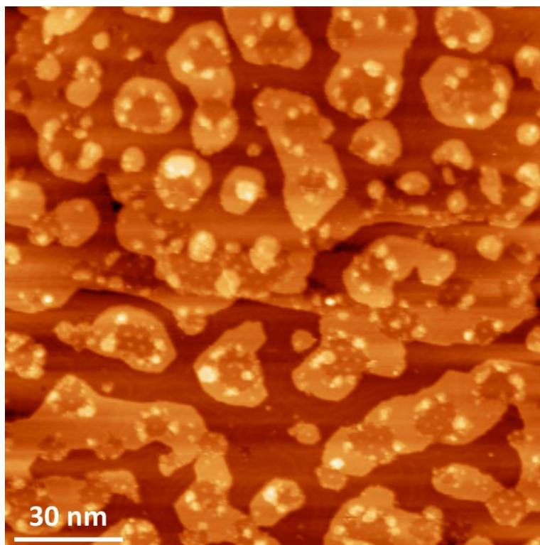
**Fig. S3** High-coverage Pd deposited on FeO/Au(111) ( $V_{\text{bias}} = 1.5$  V,  $I = 0.3$  nA). All edges of FeO islands are covered by Pd.
