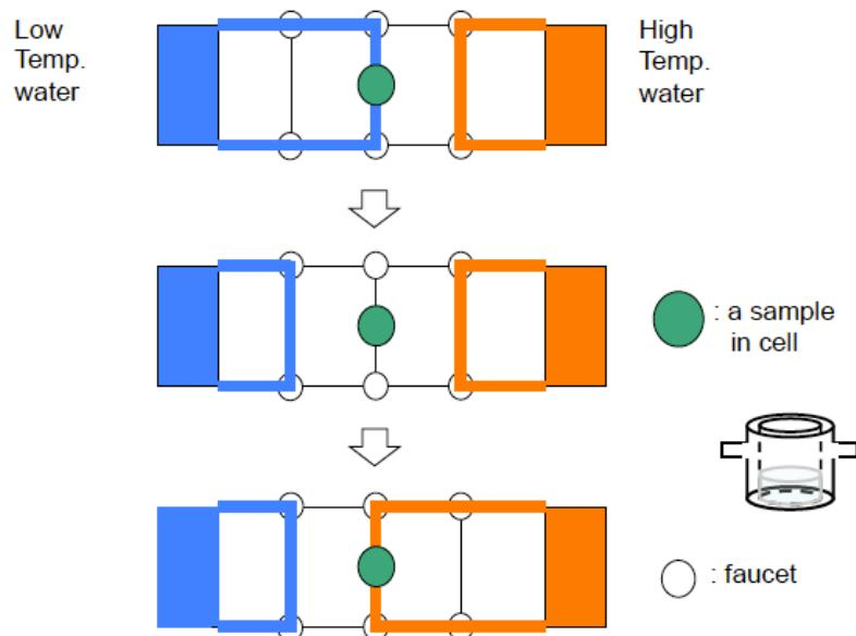
Figure S23. Circuit for temperature jump
