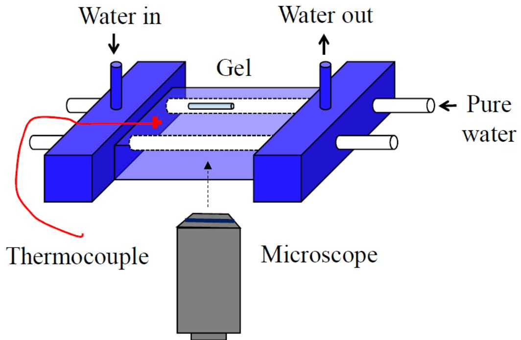
Figure S22. Illustration of equipment for swelling measurement of spherical gels
