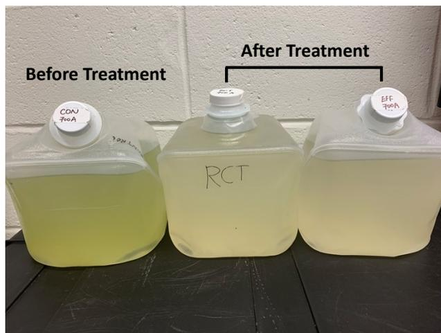
**Figure S9.** Pictures of influent and treated effluent water samples collected from the full-scale ECO treatment of Lake Neatahwanta water at a current density of  $7 \text{ mA/cm}^2$ .
