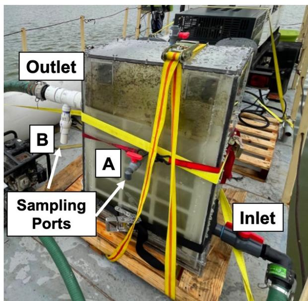
**Figure S8.** Picture of the full-scale ECO reactor. Samples from port A represent the bulk concentration in the reactor. Samples from port B are considered treated effluent.
