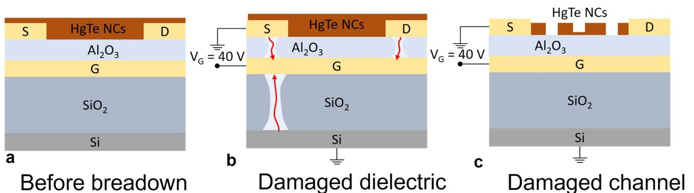
**Figure S 8** Schematic of the suggested breakdown mechanisms. *a.* Device before breakdown. *b.* Device damaged via a filamanentation through the dielectric or *c.* through a removal of the channel.
