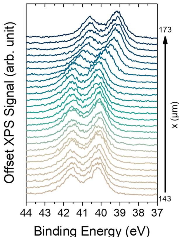
**Figure S 5** Spectra relative to the Te 4d state extracted from the map of Figure S 4, along the x axis and for a y position overlapping with the defect.
