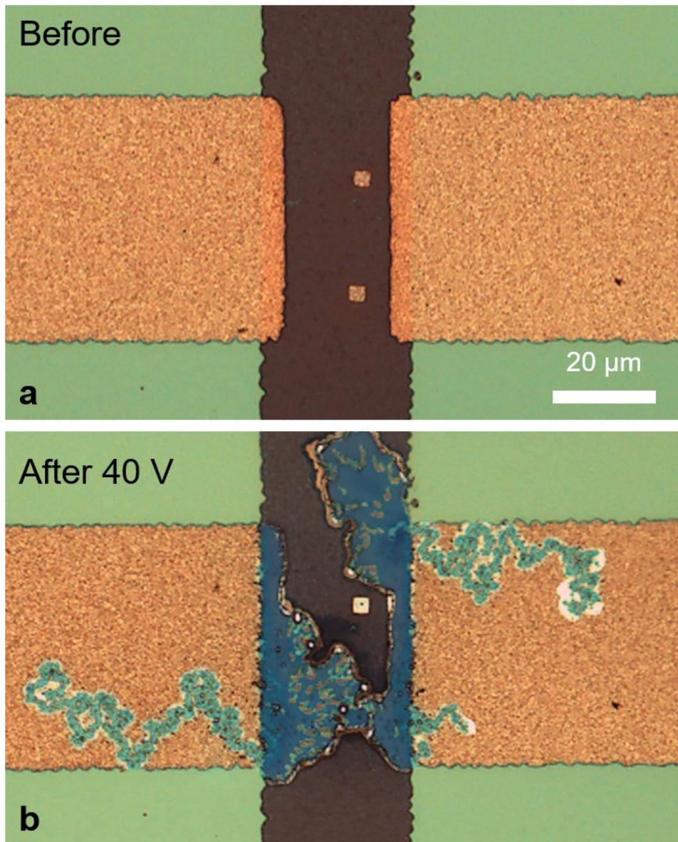
**Figure S 7** Imaging from a second FET before and after its exposure to a 40 V gate bias. *a.* (resp *b.*) Optical microcopy image from the channel of a second FET before (resp after) its exposure to a 40 V gate bias. Scale bar is the same for part *a* and *b*.
