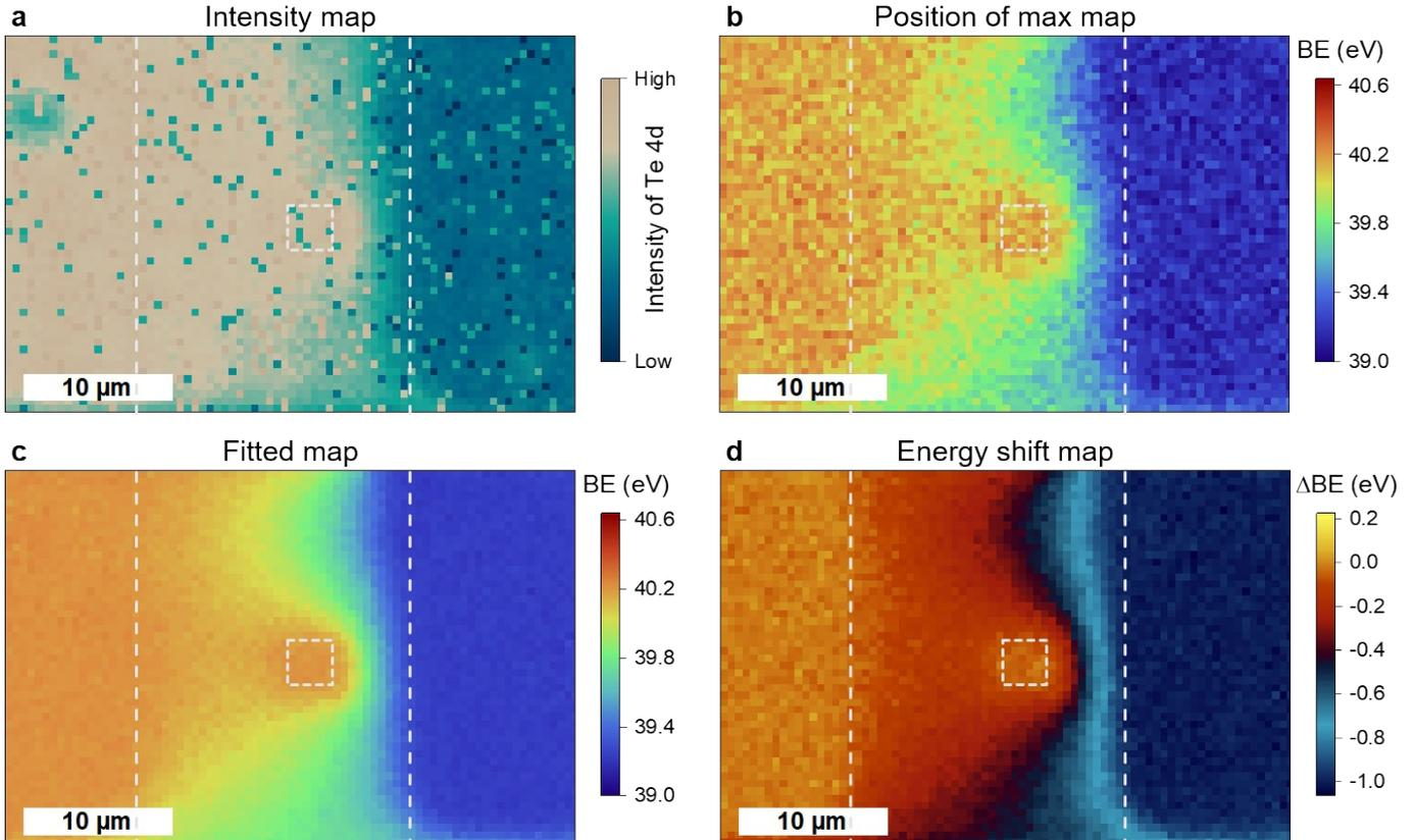
**Figure S 4** Data analysis procedure. Data are acquired while  $V_{DS} = -1$  V,  $V_{GS} = 0$  V. a. Map obtained from the integrated intensity of the Te 4d<sub>5/2</sub> component in the Te 4d spectrum. b. Map of the same
