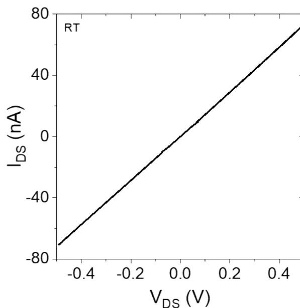
**Figure S 2 I-V curve at room temperature for the hole-free conventional FET.**
