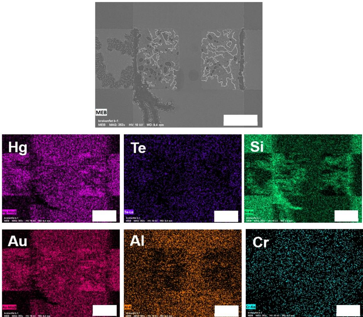
**Figure S 6. Post mortem EDX mapping.** (top) SEM image relative to the FET, described in Figure 4 from main text, after its exposure to 40 V gate bias. (bottom) EDX mapping relative to Hg, Te, Si, Au, Al and Cr. All scale bars (white rectangles) are 30  $\mu\text{m}$  long
