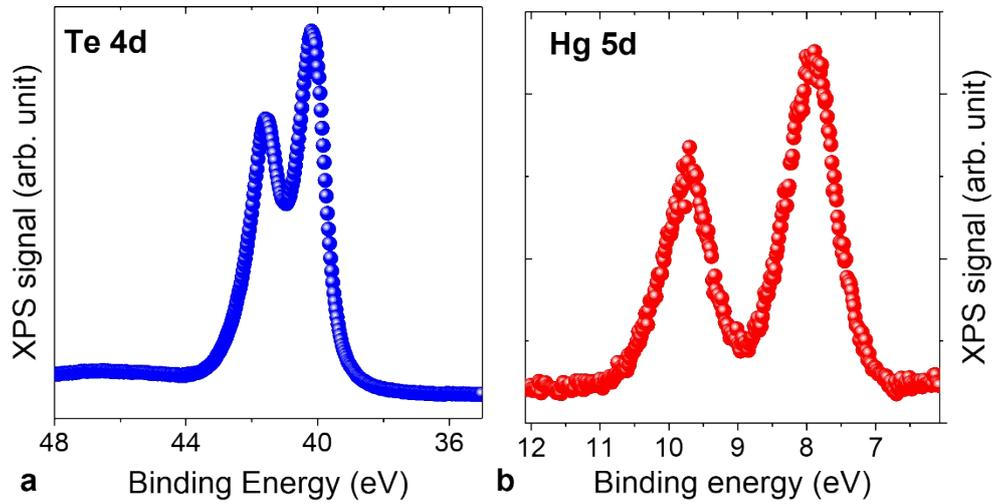
**Figure S 3** Low energy core levels from the HgTe CQD film. a. Spectrum relative to the Te 4d state. b. Spectrum relative to the Hg 5d state.
