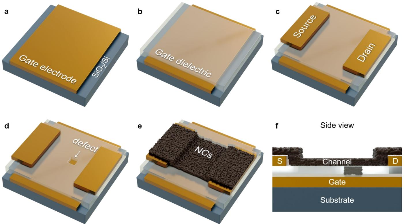
**Figure S 1 Fabrication of the defective FET.** a. Deposition of the back gate electrode. b. Deposition of the alumina used as FET dielectric. c. Deposition of the drain-source electrodes defining the FET channel. d. E-beam lithography step to etch a hole within the dielectric. e. Coating with the HgTe CQD film. f. Side view of the device from part e.
