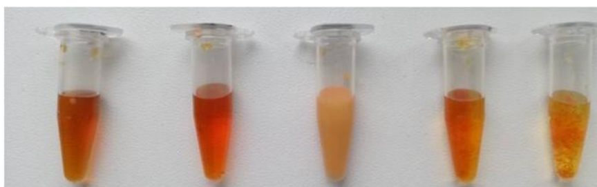
Figure SIII.1. Solutions of the studied substances, from left to right: Na-Mo 2 O 4 -EDTA , Na-Mo 2 O 4 -L-Cys , K-Mo 2 O 2 S 2 -EDTA , K-Mo 2 O 2 S 2 -L-Cys , K-Mo 2 O 2 S 2 -HNTA ; Conc. 50 mg/mL.
